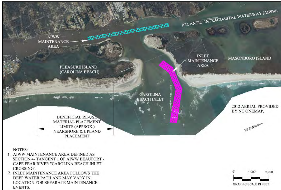
Figure 8. Carolina Beach Inlet Maintenance Areas & Beneficial Re-Use Material Placement Limits
